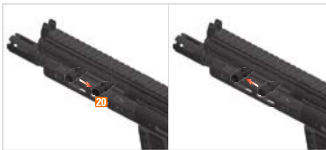
2. Pull the cocking lever 20 back until it stops and allow it to slide forward. The gun is now cocked, loaded and with safety engaged.
